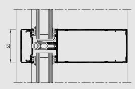
Concept Wall<sup>®</sup> 50 is a façade and roof system that offers unlimited design freedom and allows maximum transparency. As such, CW 50 meets all requirements of contemporary architecture. Innovative solutions contribute towards the tendency of big, heavy and thick glass panes. CW 50 supports up to 150, 310 and even 600 kg in various glass support configurations.
